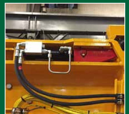
Wedge lock secures upper hog box
