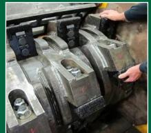
Steel drum rotor with twenty 6" x 8" steel striker plates held in place by two 1-1/4" bolts, designed for contaminated demolition debris, railroad ties, and MSW.
